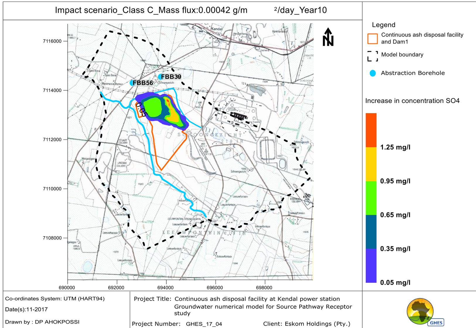
Figure 34: Simulated pollution plume impact for Intermediate Class C liner after 10 years
