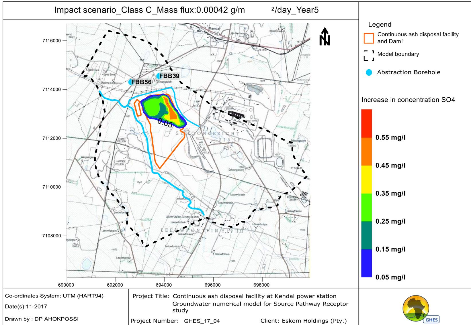
Figure 33: Simulated pollution plume impact for Intermediate Class C liner after 5 years
