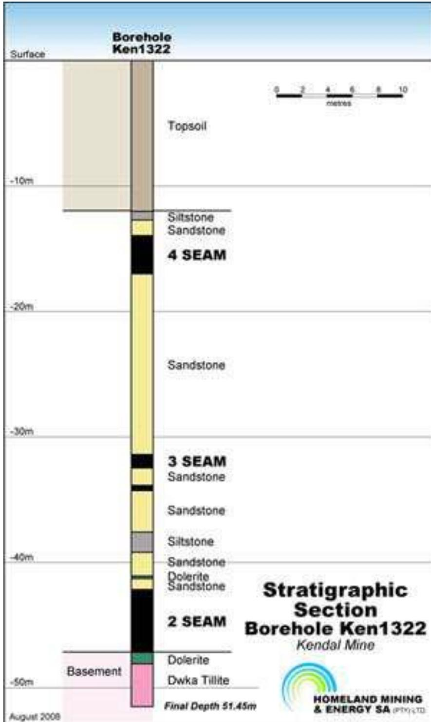
Figure 6: Typical stratigraphic section at KPS (Homeland Mining & Energy SA)
