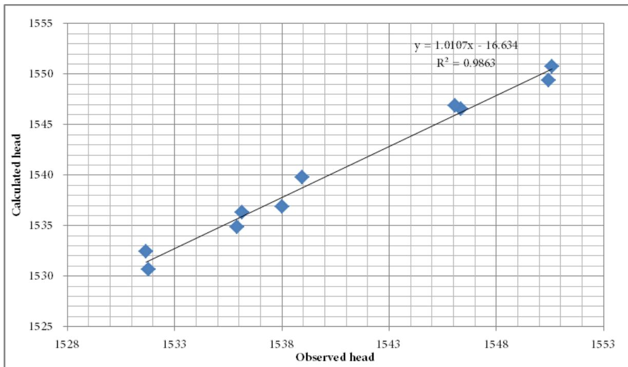
Figure 28: Observed versus calculated groundwater elevations
