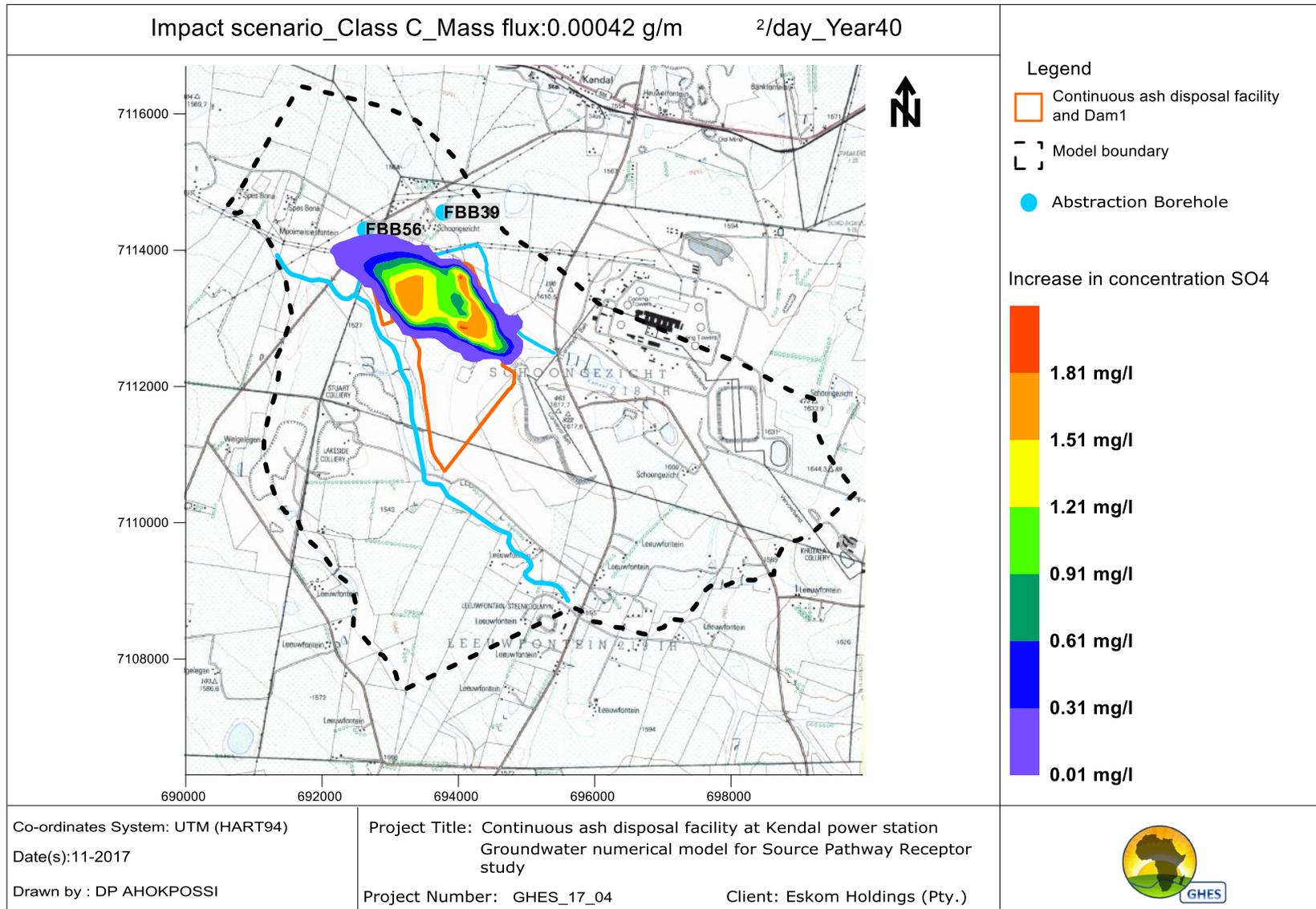
Figure 35: Simulated pollution plume impact for Intermediate Class C liner after 40 years
