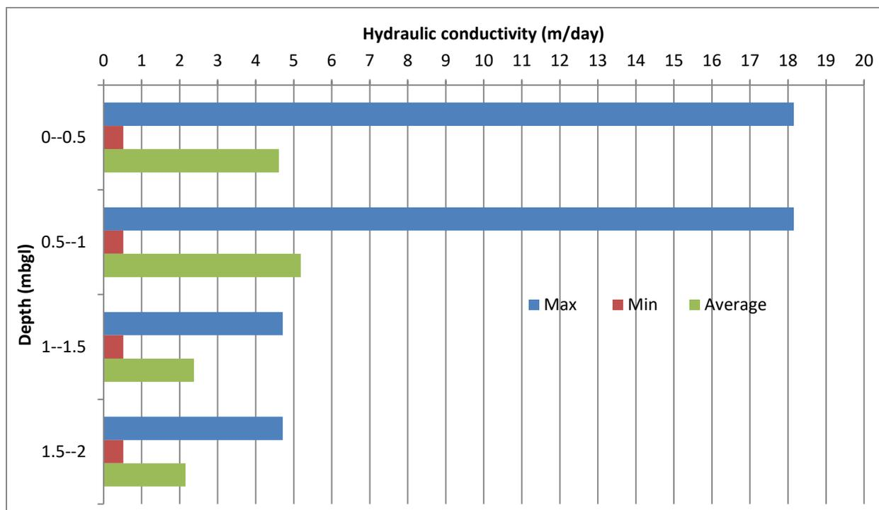
Figure 23: Vertical distribution of recorded conductivity in the soil
