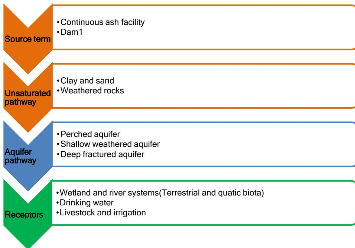
Figure 24: Link between source-term, groundwater and receptor studies
