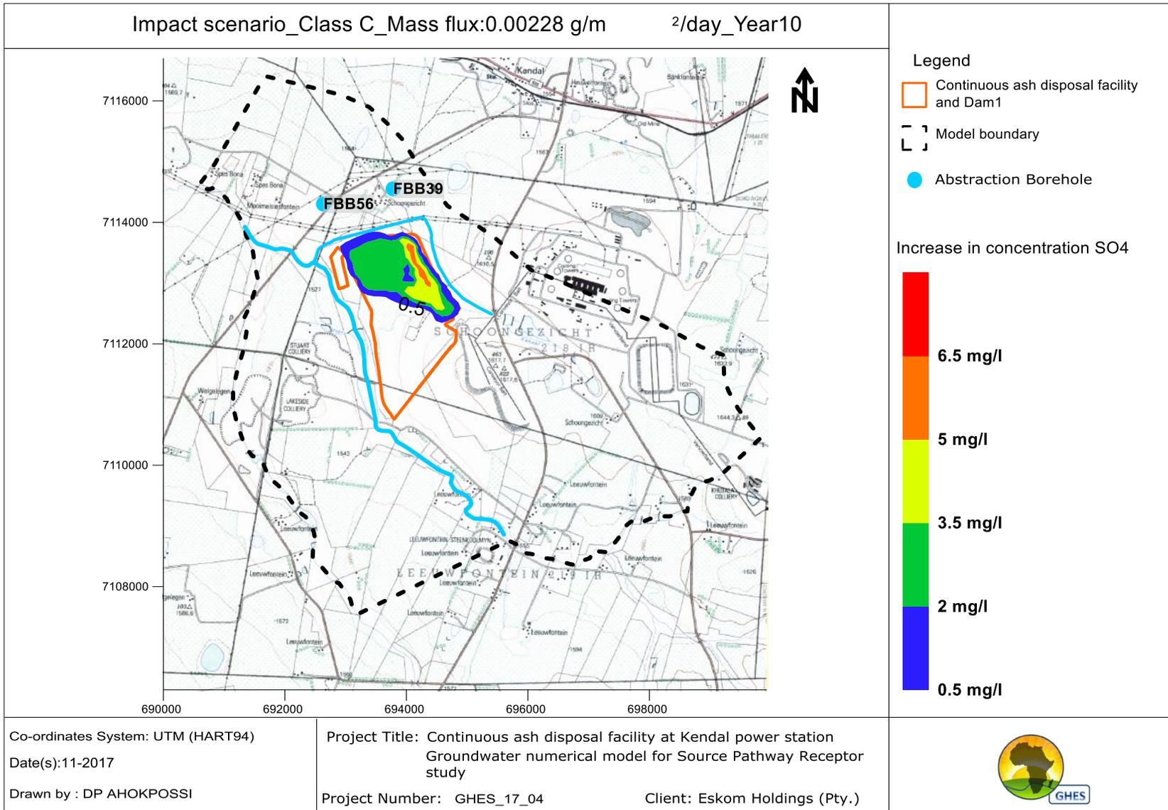
Figure 31: Simulated pollution plume impact for Class C liner after 10 years
