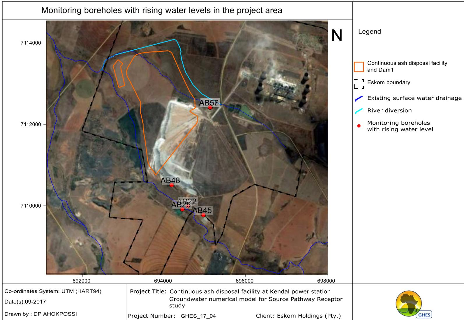
Figure 12: Monitoring boreholes with rising water level
