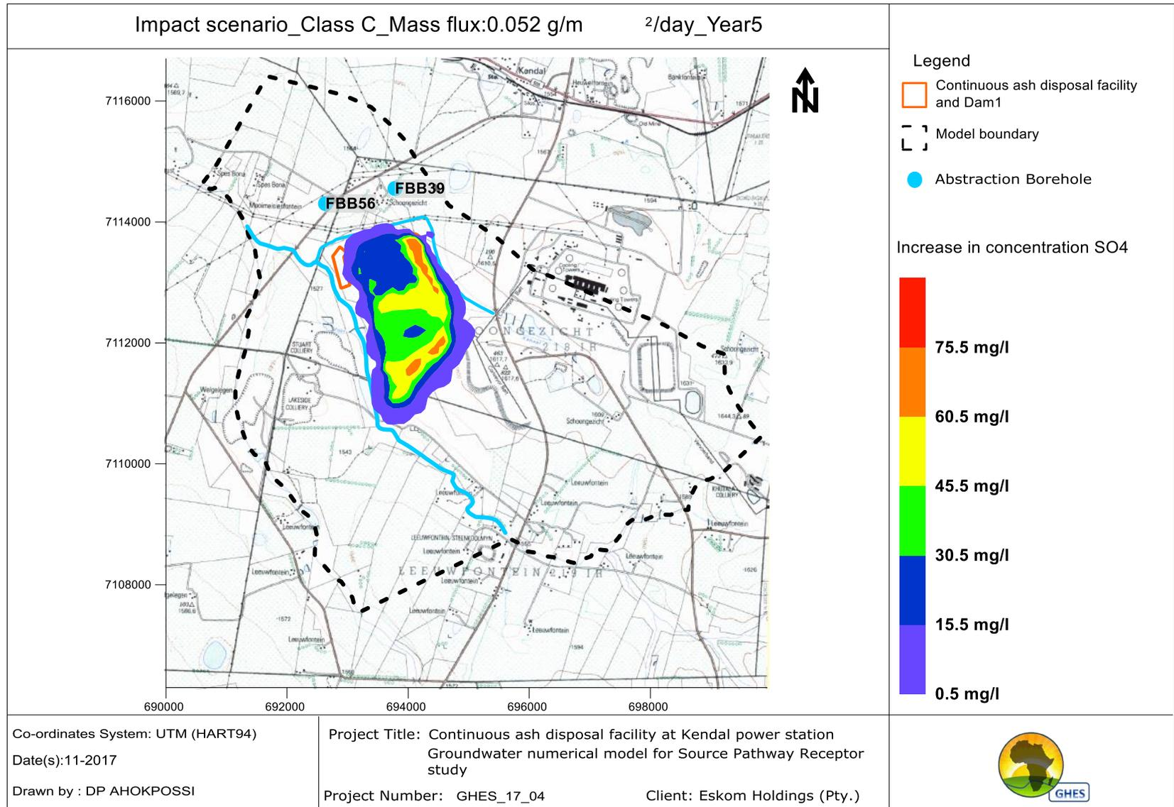
Figure 36: Simulated pollution plume impact for Class D liner after 5 years
