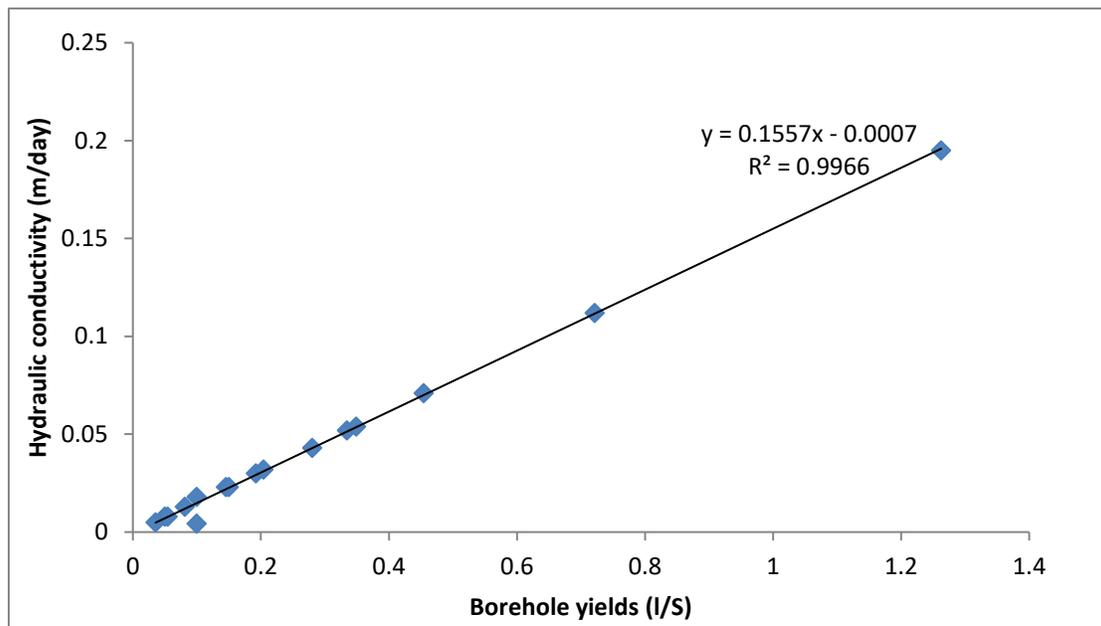
Figure 22: Correlation between recorded hydraulic conductivity and borehole yields (for values above 0.036 l/s and 0.005 m/day)
