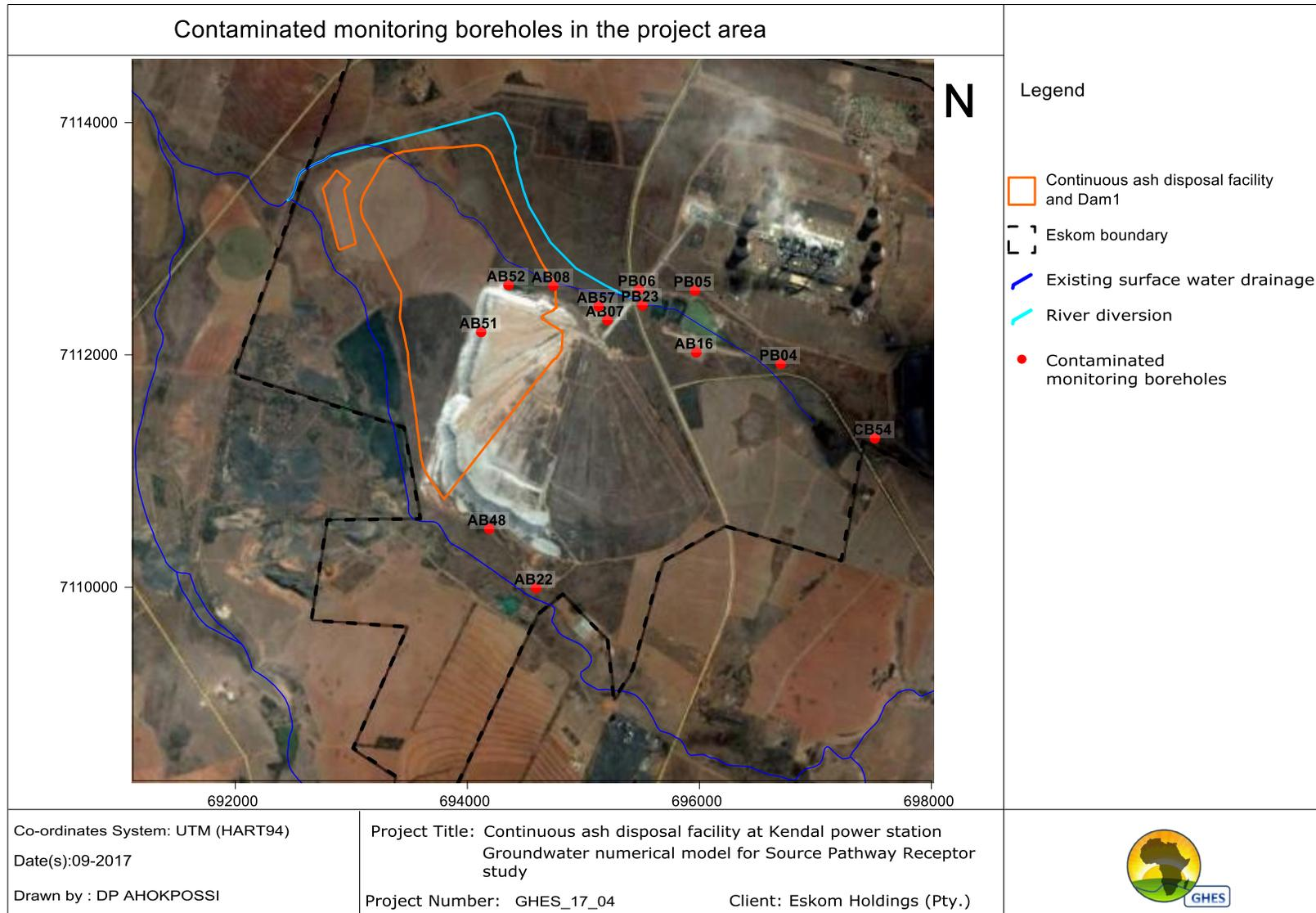
Figure 11: Contaminated monitoring boreholes in the project area
