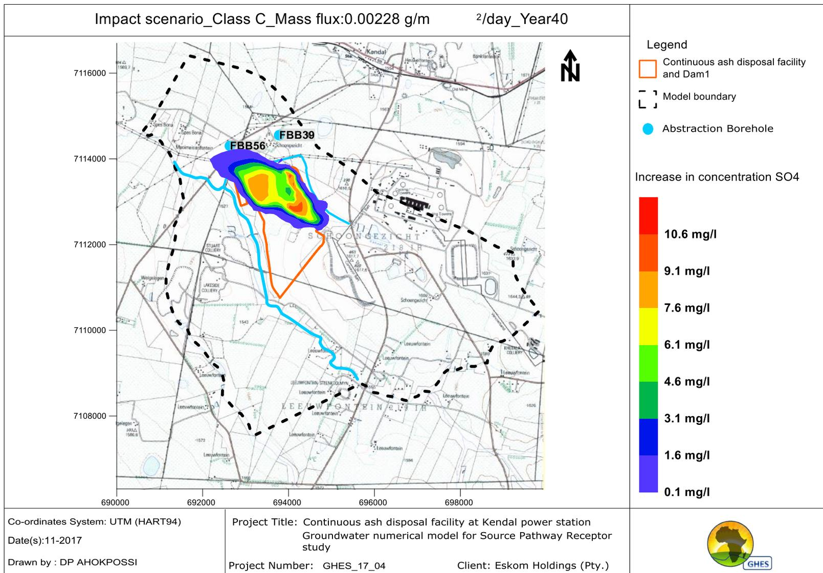
Figure 32: Simulated pollution plume impact for Class C liner after 40 years
